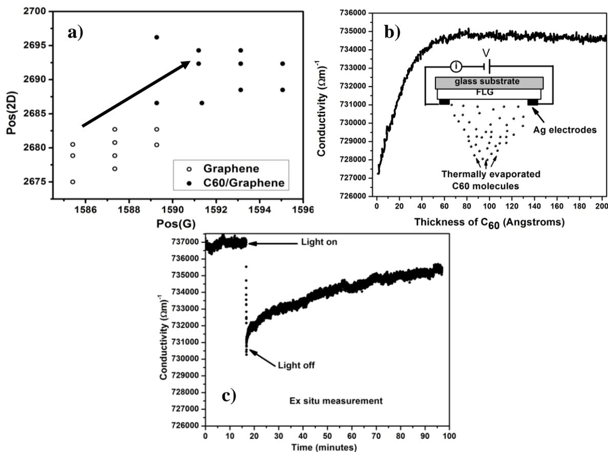
a) Position of G and 2D peaks of graphene with and without thermally evaporated fullerene  $C_{60}$ ; b) Conductivity of FLG film versus thickness of  $C_{60}$  in darkness; c) Behavior of electrical conductivity of FLG film with  $C_{60}$  under illumination; for this experiment we used a 514.5 nm of laser excitation and 10 mW of Intensity.
